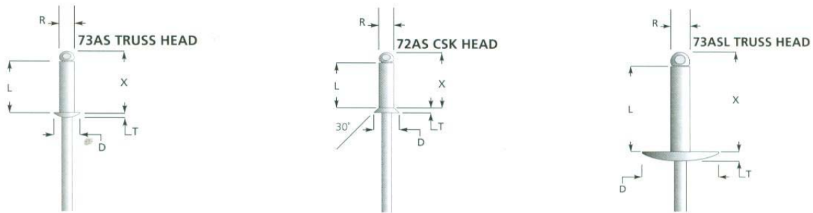
Figure 5b-2. Blind rivets have three basic head styles.
